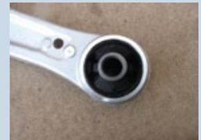
2008 Subaru Impreza Sti front control arm. Note profiled rubber voids to help articulation
