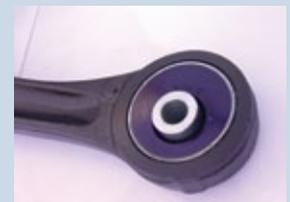
Audi TT Mk1 front control arm with SuperPro bush fitted. Note gap between bush and centre tube.
