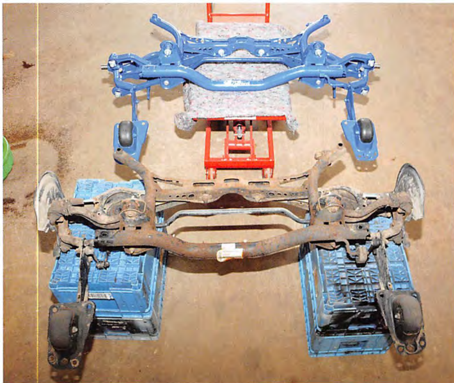
It's easy to see here just how comprehensive the SuperPro Handling Kit is and what's involved in getting the whole lot fitted. The difference it makes to the Mk5's chassis is incredible, both on the road and the track
